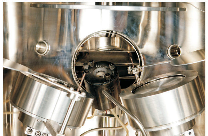
ATS 500 chamber with two 100mm sputter sources & ion beam source
