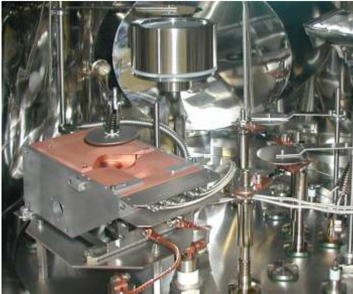
TF600 chamber with 6kW electron beam source, 4" sputter source and two 2kVA resistance sources
