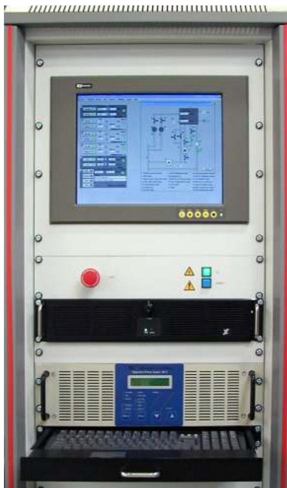
TF600 rack with PC control for fully automated system and process operation
