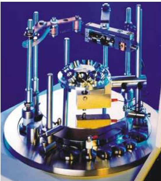
Auto306 by resistance and carbon sources for SEM. The Rotatilt3 work holder is fitted by the SEM planetary sample holder
